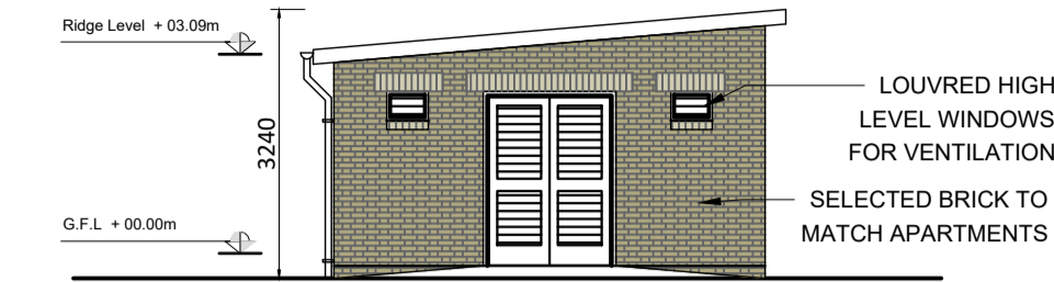
Block D Bin Store - South-west Elevation
