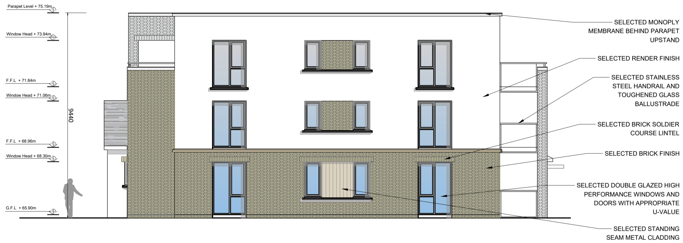
Block D - South-east Elevation
